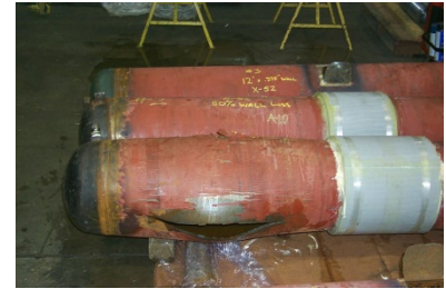
Pipe Body Failure @ 4,260 psi
